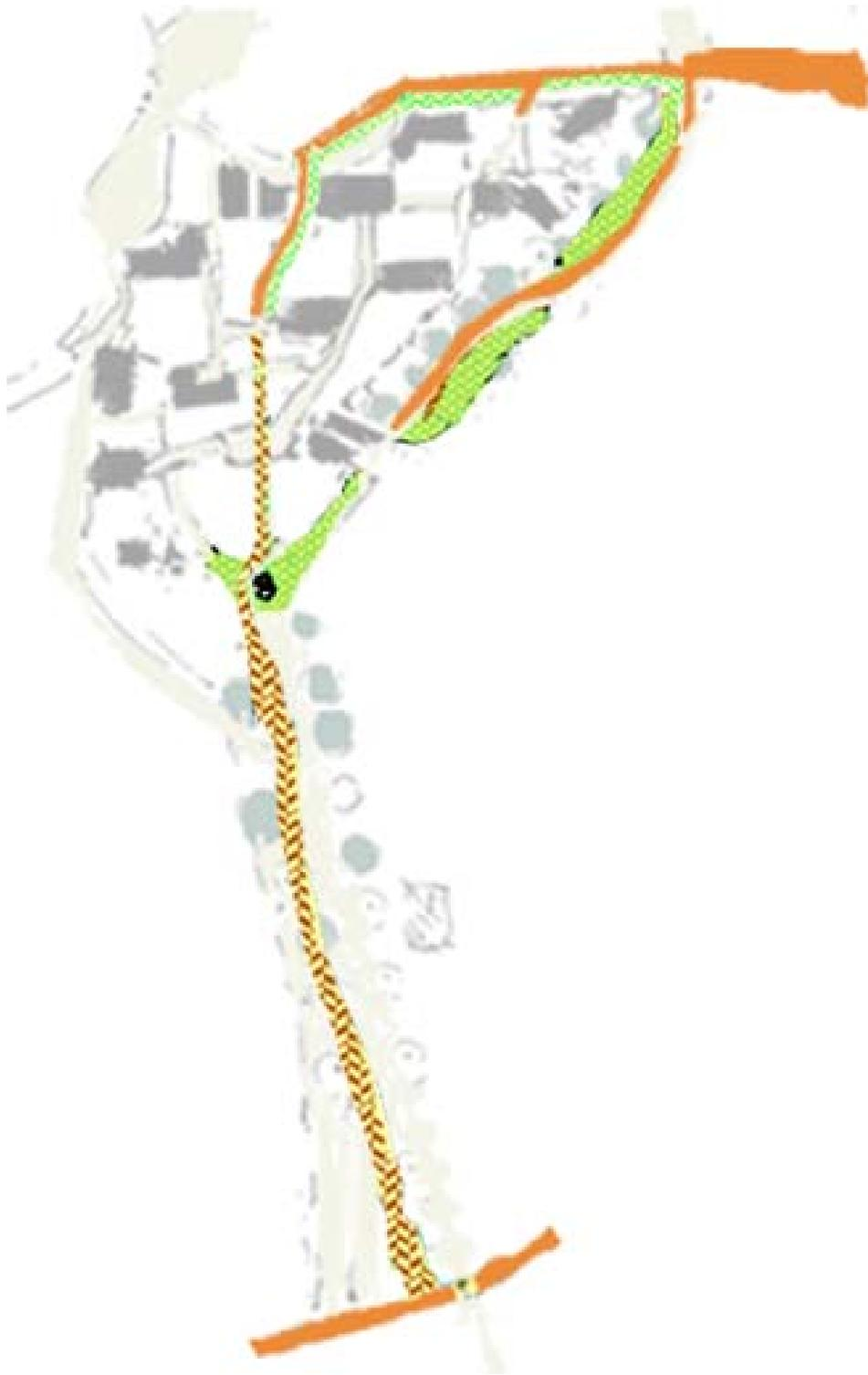
*Step 8.7. The process of introducing grass block and reinforced turf along the shoulders of local roads as a breakdown lane, pleasant to look at and to walk on, but capable of taking the weight of firetrucks and other heavy vehicles in all weather conditions.*
