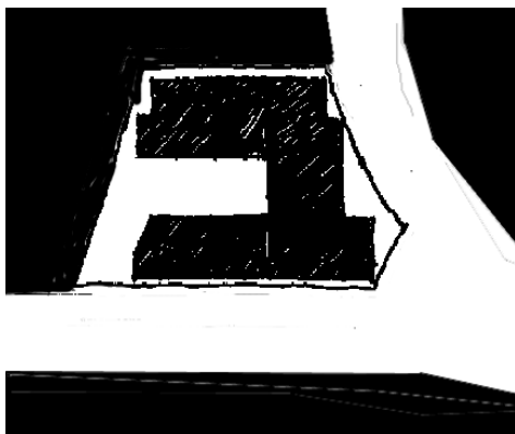
Left: On the left, a first possible site plan, rather conventional in character, which is NOT structure preserving. Although this plan follow typical building and design character for a building in the 1970's or 1980's, the placing of the volumes, the badly formed exterior space, and the lack of structure-preserving impact on the two streets and on the sunshine in the south, are all negative. Right: The building site plan as we actually built it, showing the unusual building configuration caused by the fork, and two bent streets, Christopher Alexander, Hajo Neis, Ingrid King, 1987
