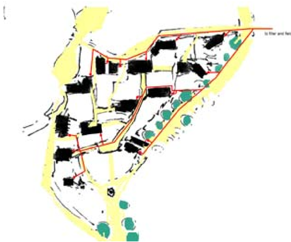
Step 8.13. Sewer lines shown in red. The total cost per house of these small bore sewers is less than the cost of main sewer lines for a typical, conventional, group of houses in a tract.
