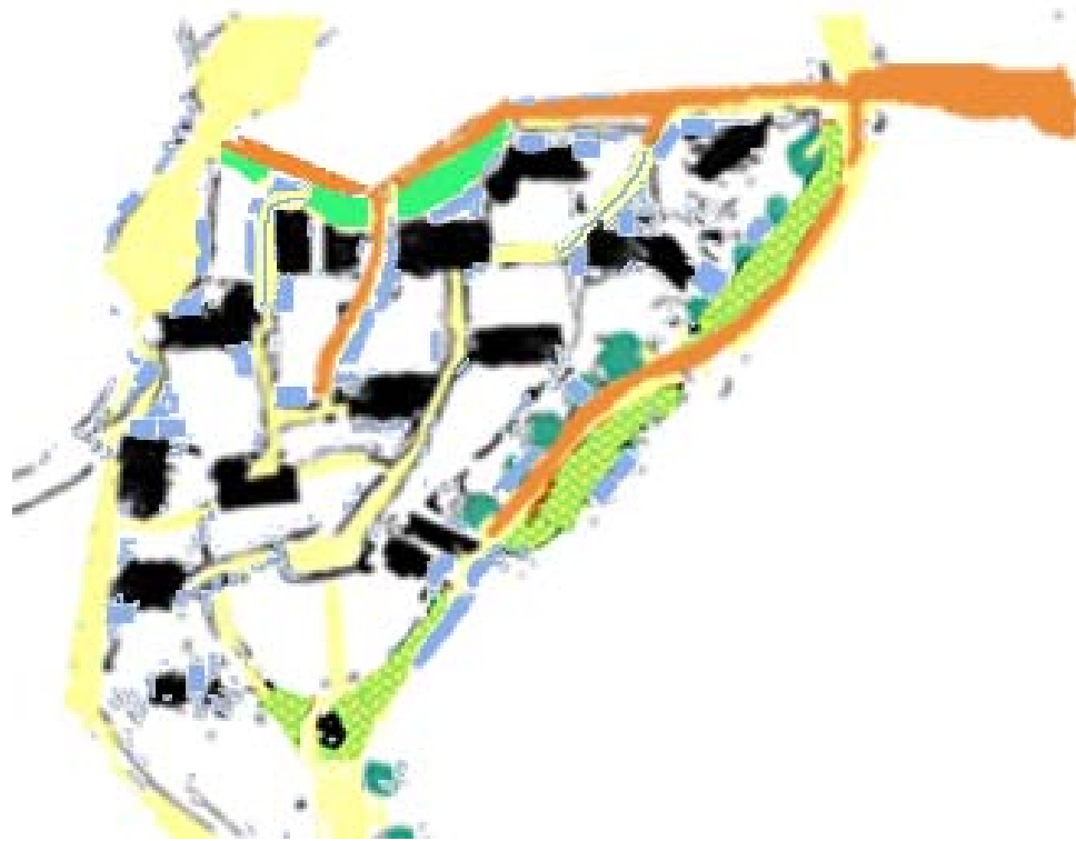
Step 8.10. The drives and lanes needed to reach all those parking spaces not directly accessible from the local road, are shown as a yellow path with a thin blue line down the middle.
