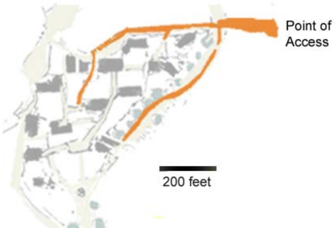
Step 8.5. Point of Access, showing the process of introducing local roads, shown in red, as they fan out from the point of access. The black bar shows the dimension of 200 feet, and allows one to see that in this neighborhood, only two houses (as permitted) are more than 200 feet from the local roadway.
