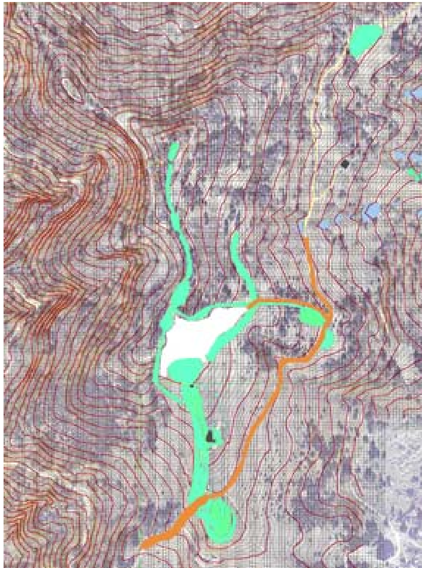
Step 8.4. The principle point of access for the new neighborhood, shown in red. The upper right hand road comes in to the neighborhood from the major North-South collector, and requires the least new road construction, while preserving existing structure by using the alignment of a logging trail.
